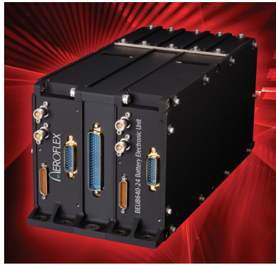
Fig. 2. Dual redundant BEU targeting 24-cell battery applications.
