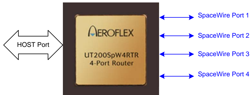
Figure 14. 4-Port Router configuration for the look up table access and configuration example
