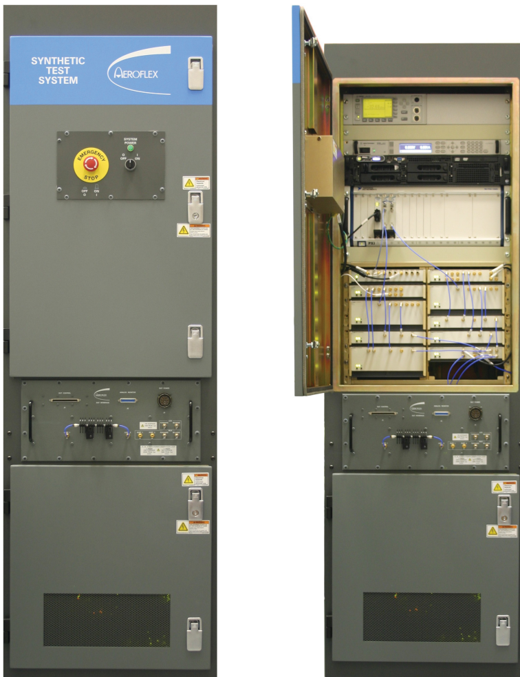
Figure 4. Shown is the exterior and interior of Aeroflex's synthetic test environment, which can support a number of standards thanks to its hybrid integration capability.
