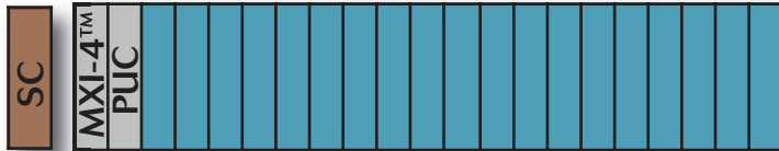
21 Slot Common Core Backplane
